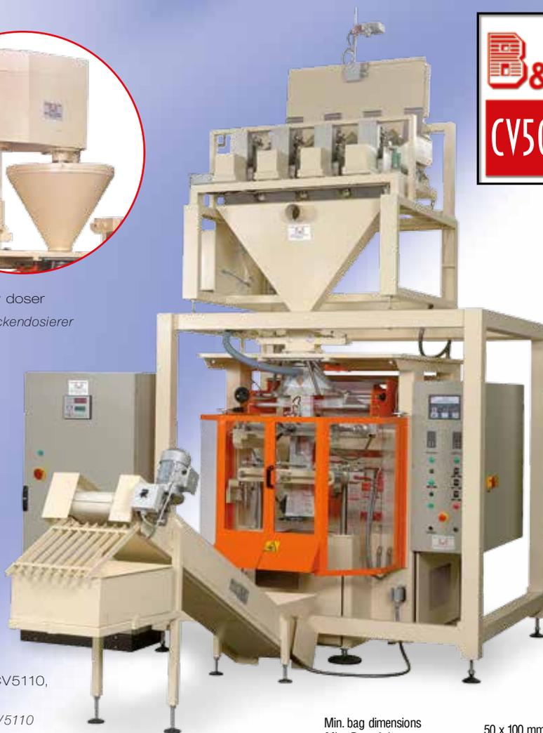
Form/fill/seal machine Mod. CV5110,
